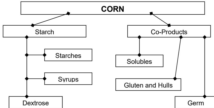
Upon arriving at a processing plant, each load of corn passes through a cleaner that removes foreign material and other impurities. Then the corn is soaked for 36 to 48 hours in hot water and sulfur dioxide. This process softens the protein (gluten) within the starch matrix while also toughening the germ.
